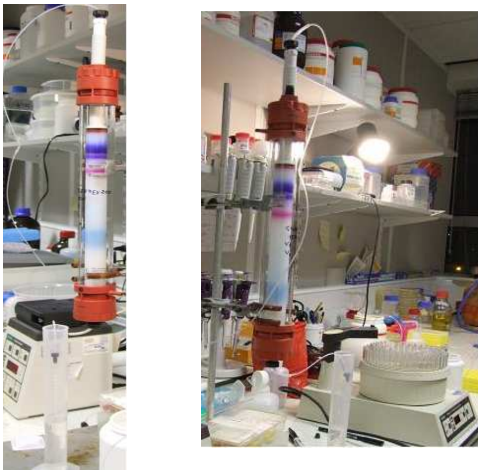
Figure 2.9 Experimental measure of the void volume in the gel filtration column
