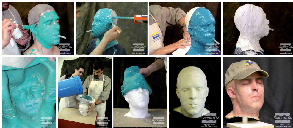
Silicone Rubber to Make a Mold of a Head @ http://www.smooth-on.com/
