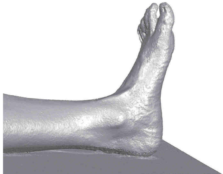
Virtual reconstruction of the lower limb surveyed with Konica Minolta Non-contact 3D digitizer Vivid 910
