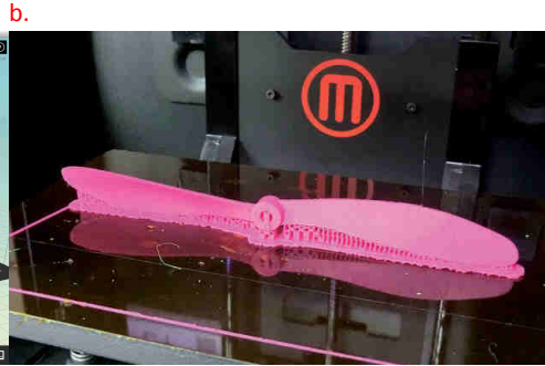
a. and b. 3D-printed propeller for model airplane @Creative Tools https://www.flickr.com/photos/creative_tools/9155457179
