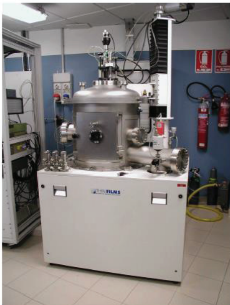
Fig.4.10. Plasma Sputtering Equipment. Off-axis rotating system to improve the film thickness uniformity (A). Magnetron sputter gun (B).
