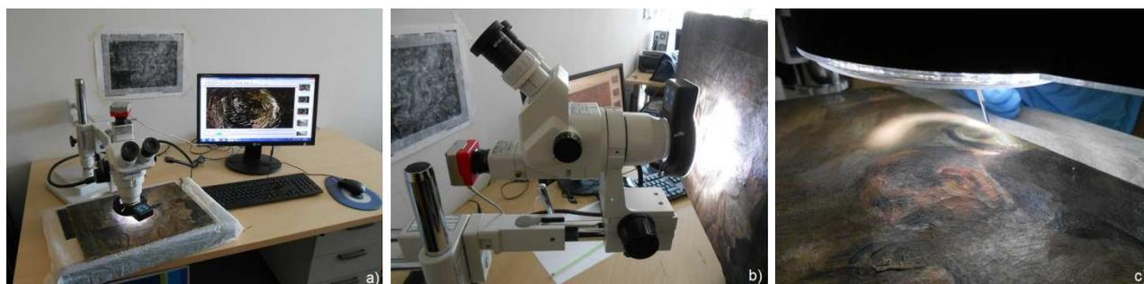
**FIG. 16** Stereomicroscope OPTIKA SZ6745TR (Physics and Earth Science Department, Ferrara University, Italy): a) horizontal working set up; b) vertical working set up; c) sampling on artwork “Reader woman on bed and old man” (artwork plate IV) under stereomicroscope.
