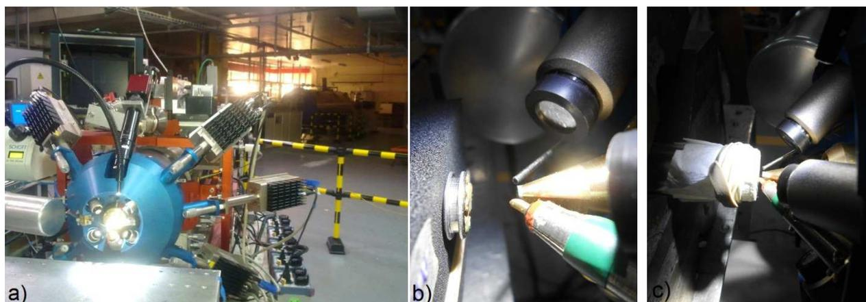
**FIG. 19** AGLAE facility (Centre de Recherche et de Restauration des Musées de France, Palais du Louvre, Paris – France): a) AGLAE, external microbeam used to perform PIXE analysis; b) PIXE analysis on samples placed on stub (specimens taken from studied Modigliani’s artwork); c) PIXE analysis on free samples placed on filter in hand-made vacuum system (specimens taken from “Flowers” by F. De Pisis).
