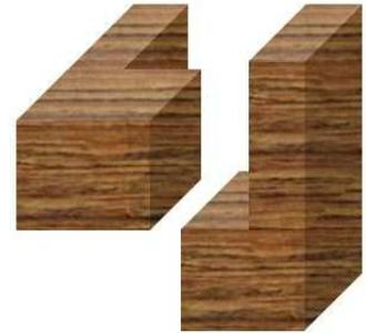
**FIG. 138** Schema of possible “L” joint in studied painting.
