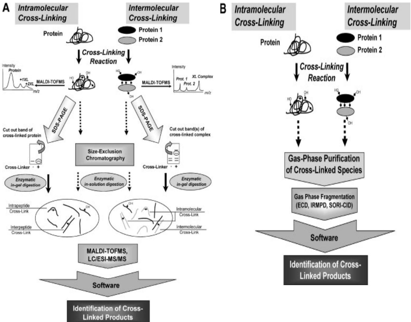
General analytical strategies for protein structure characterization by chemical cross-linking and mass spectrometry. (A) Bottom-up approach, and (B) top-down approach using FTICR-MS.
