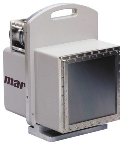
Figure 2.5. Detail of a MAR-type CCD detector (in the image the model no. 225).
