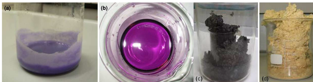
Figure 2.2. Effect on gel stability of the citrate-metal cations ratio. Stoichiometric ratio (a), stable and transparent gel achieved with an excess of citrate (b), and pictures of powders combusted at different temperatures: 300 °C (c) and 500 °C (d).
