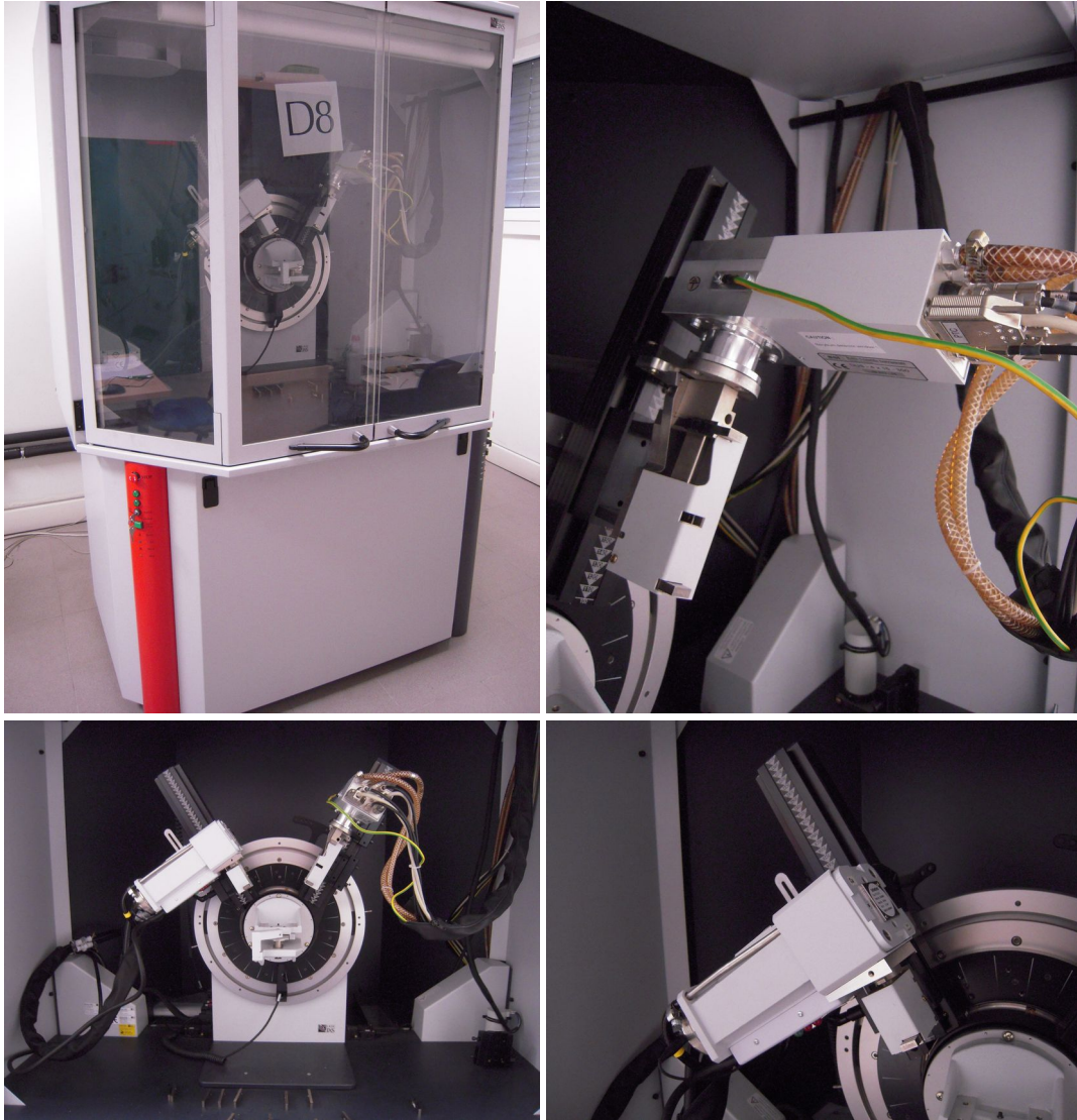
Figure 2.3. On the left, panoramic (top) and detailed (bottom) views of the Bruker D8 Advance diffractometer with a \theta : \theta Bragg-Brentano geometry settles at the department of mineralogy, petrology and geophysics of the university of Ferrara. On the right, detail of the Bruker Sol-XE energy dispersive X-ray Si-solid state detector (top) and external box of the X-ray tube (bottom).
