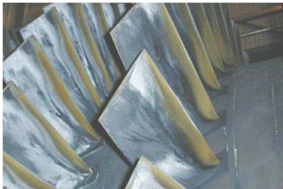
Figure 1.23 – Low Solubility Deposits on Compressor Blades (Kurz et al. , 2012)
