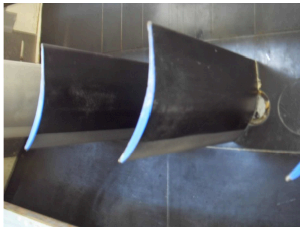
Figure 1.27 – Suction side partially covered (20 %) by a paint/glue (Back et al. , 2010)
