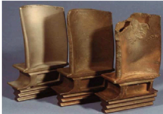
Figure 1.20 – Hot corrosion on turbine blades after about 1,000 h of operation on distillate fuel containing 2 ppm sodium from sea water contamination (Kurz et al. 2012)
