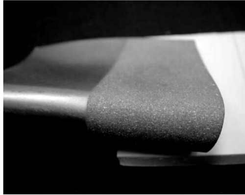
Figure 1.21 – Vane subjected to 1,500 \mu\text{m} particles, 91.4 m/s (300 ft/s), 30° incidence. Erosion rate 5 mg/g of particles (Hamed et al. , 2005)
