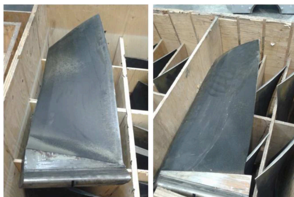
Figure 1.28 – Compressor first rotor blade visual appearance after 25,000 operating hours, pressure side on the left and suction side on the right (Silingardi et al. , 2013)
