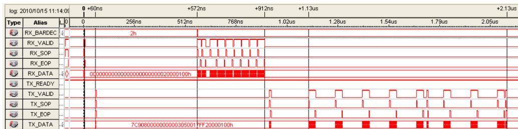
**Figure 5.9:** Timing of the NGET operations traced inside the FPGA.
